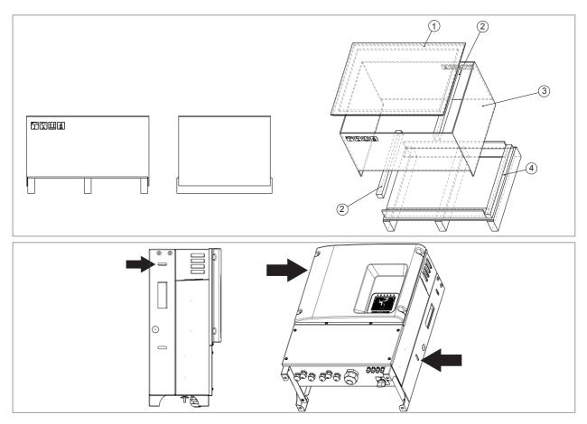
Figure 2 : wooden crate and slots for extraction of the inverter from crate
