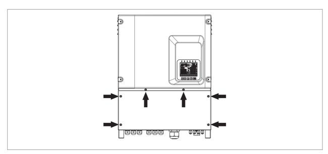
Figure 21 : Fixing of the lower panel
