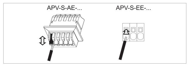
Figure 18 : Insertion of cables in spring connectors
