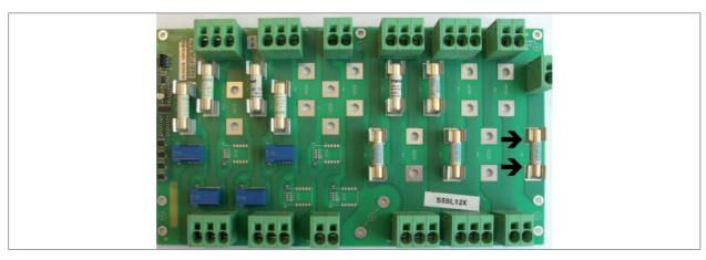
Figure 24 : Ground kit fuse (-F models)
