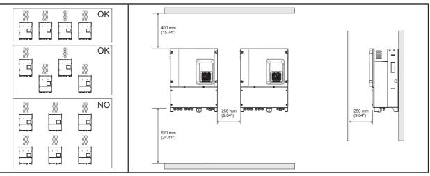
Figure 10 : Free movement of ventilation air and Minimum distances
