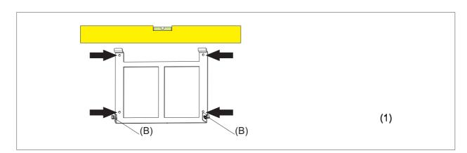
Figure 12 : Mounting bracket fixing
