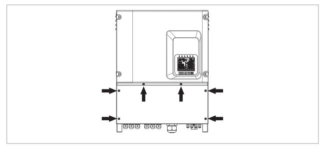
Figure 15 : removal of the lower panel
