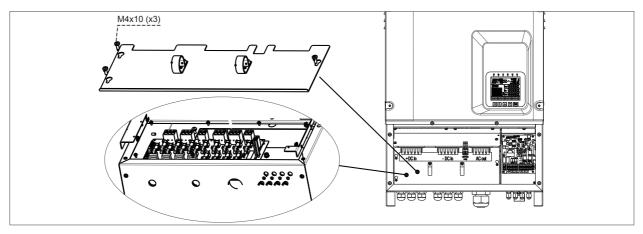
Figure 23 : DC side fuses series PVSA-..k-AE
