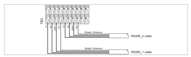
Figure 31 : RS485 connection wiring diagram (example)
