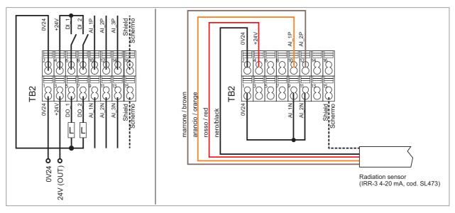
Figure 30 : Regulation circuit Input/Output connection diagram (example)
