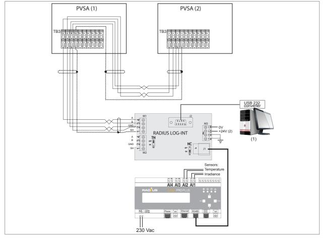
Figure 35 : Example of connection with multiple inverters
