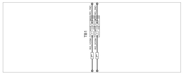
Figure 29 : Relay output wiring diagram (example)
