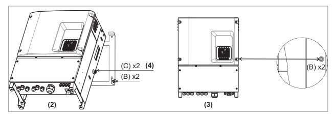
Figure 13 : Fixing the inverter on the bracket
