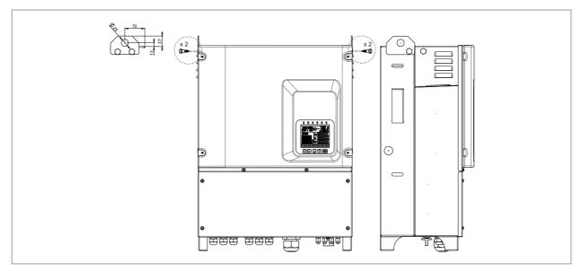
Figure 3 : Mounting of transport brackets for handling with hoist
