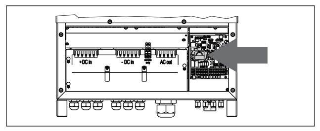
Figure 38 : Position of battery on electronic card
