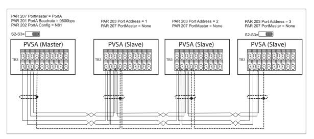
Figure 37 : Example of M/S connection
