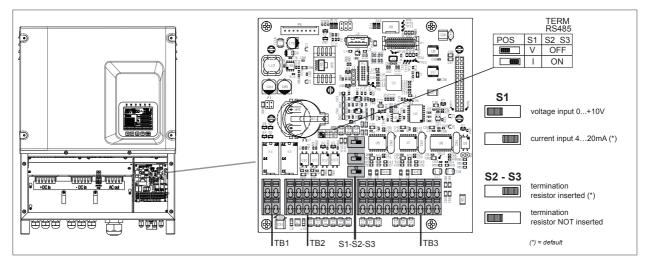
Figure 27 : Regulation and communication terminals. S1-S2-S3 switches
